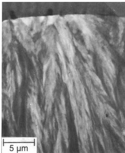
Figure 6 Same sample as in Figures 4 and 5 but lower magnification. Fibrills of the transcrystalline regions of i -PP46k can be seen.
